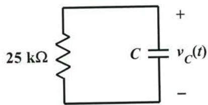
$$\frac{1}{(25\text{k}\Omega)C} = 8 \Rightarrow C = \frac{1}{8(25\text{k}\Omega)} = 5\mu\text{F}$$
