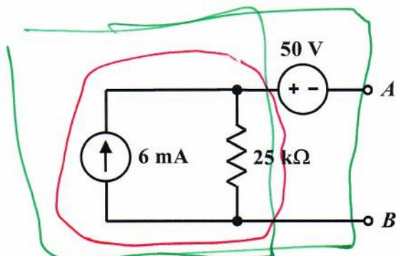
Find the Thévenin equivalent circuit with respect to terminals A and B.
