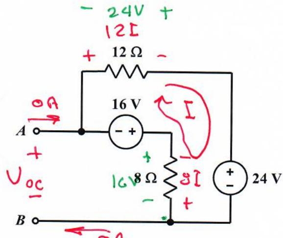
Find the Thévenin equivalent circuit with respect to terminals  $A$  and  $B$ .
