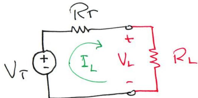
What value of  $R_L$  will absorb maximum power from the circuit?
