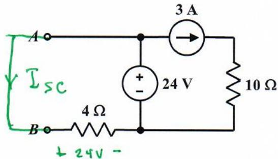
Find the Norton equivalent circuit with respect to terminals A and B.
