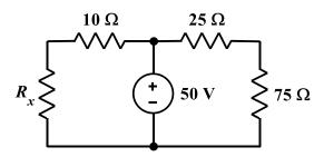
(a) What value of  $R_x$  will absorb maximum power from the remainder of the circuit?
