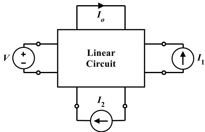
$I_o = 20 \text{ mA}$  when  $V = 2 \text{ V}$ ,  $I_1 = 0 \text{ A}$  and  $I_2 = 2 \text{ A}$ .
