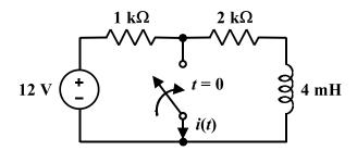
6. The circuit shown below has reached the DC steady-state prior to t = 0.
